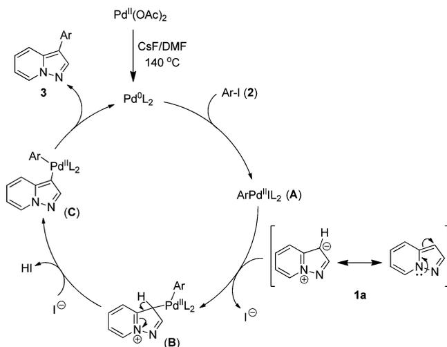
**Figure 2.** Proposed mechanism for the direct C-3 arylation of **1a**.
