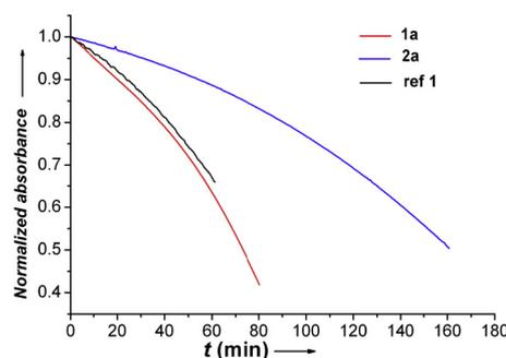
Fig. 5. Normalized absorbance of photochromic compound under continuous irradiation with xenon lamp.
