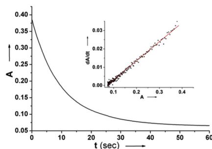
Fig. 4. Thermodecoloration of Closed-TC of compound **1a** in toluene ( $5 \times 10^{-5}$  M) at 298.4 K monitored at 478 nm. Inset: linear fit.
