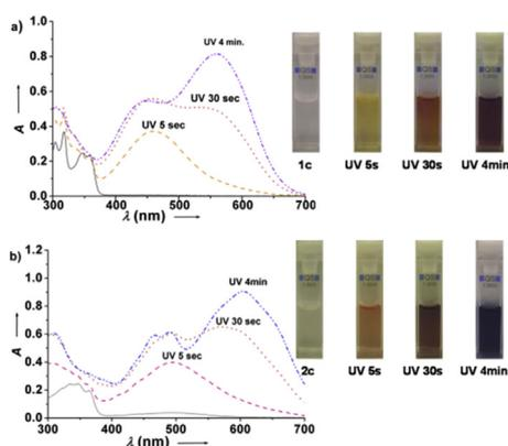
**Fig. 1.** UV–visible spectra of  $2.5 \times 10^{-5}$  M solution of bispyran **1c** (top) and **2c** (bottom) prior to and after UV (366 nm) irradiation at room temperature, respectively.
