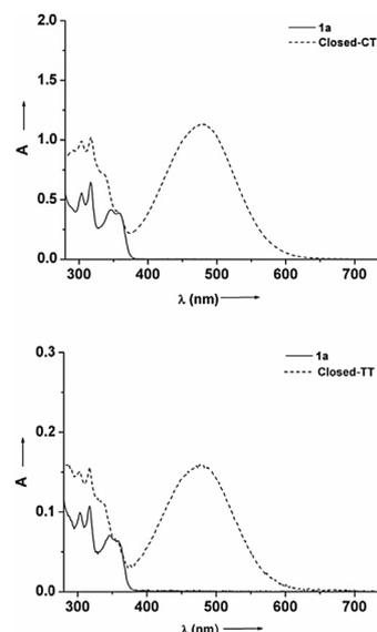
**Fig. 2.** Absorption spectra of the colored species of **1a** isolated by low-temperature chromatography on silica gel at  $-78$  °C in dichloromethane.
