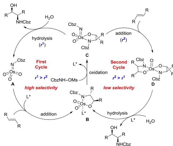
Scheme 1. First and Second Cycles of the SAA reaction.
