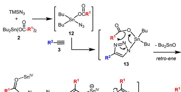
**Scheme 5.** A plausible mechanism for the conversion of dibutyltin diacylates **2** to 2,4-disubstituted oxazoles **4**.
