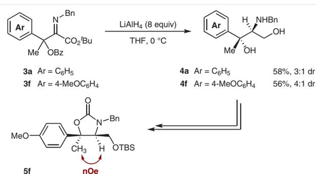
**Scheme 3** LiAlH<sub>4</sub> reduction of products **3a** and **3f** and determination of diastereoselectivity via NOESY experiments with the derived cyclic carbamate **5f**
