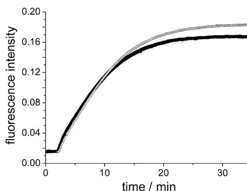
**Figure 1.** Fluorescence–time plots for the reaction of **8b** (gray) and **8c** (black;  $1.0 \times 10^{-6}$  mol L<sup>-1</sup>) in methanol containing pyridine ( $1.0 \times 10^{-4}$  mol L<sup>-1</sup>) with hydrogen.
