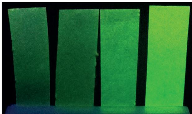
**Figure 2.** Four filter paper strips (left to right: a–d) impregnated with a solution of **8b** in propylene carbonate and irradiated with broadband UV light. Strip (a) exposed to ambient air; strip (b) exposed to 1% (vol) H<sub>2</sub>; strip (c) exposed to 4% (vol) H<sub>2</sub> (lower explosion limit), and strip (d) exposed to pure H<sub>2</sub>.
