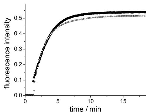
**Figure 4.** Emission–time plot for the catalytic hydrogenation of 0.1 M allylbenzene (gray) with **8b** (black;  $1.0 \times 10^{-5} \text{ mol L}^{-1}$ ) in 1,2-dichloroethane; same reaction conditions, but without olefin (black).
