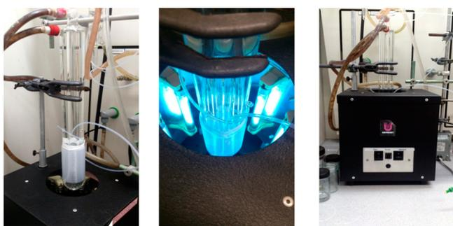
Figure 1. Small scale photochemical flow reactor.
