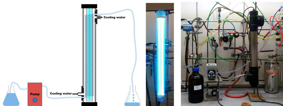
Figure 2. Large scale photochemical flow reactor: schematic overview and complete setup.
