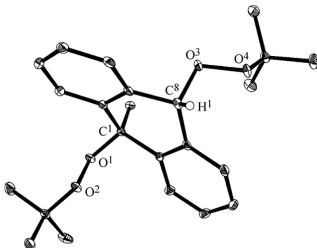
Fig. 1. Molecular structure of 9-methyl-9,10-dihydro-9,10-di-*tert*-butylperoxyanthracene (**II**).
