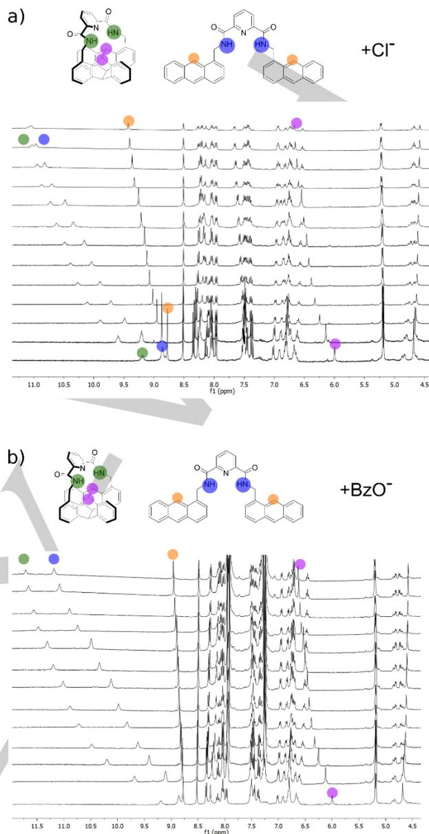
**Figure 4.** Competitive  $^1\text{H}$  NMR titrations of a mixture of **10** and **11** with  $\text{Cl}^-$  (a) and  $\text{BzO}^-$  (b). The relative shift of protons of the two hosts is used to calculate the ratio of association constants.
