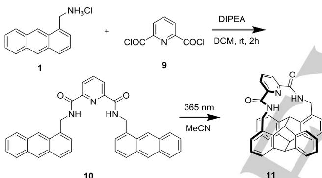
**Scheme 2.** Synthesis of receptor **10** and its transformation into **11**.
