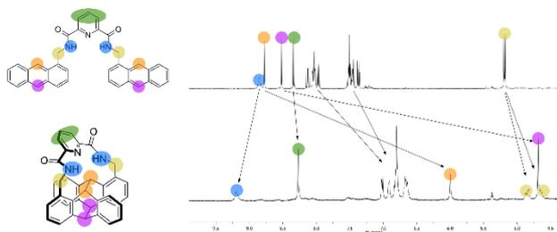
**Figure 3.**  $^1\text{H}$  NMR spectra of **10** before and after irradiation with a 365 nm lamp ( $\text{CD}_3\text{CN}$ ).
