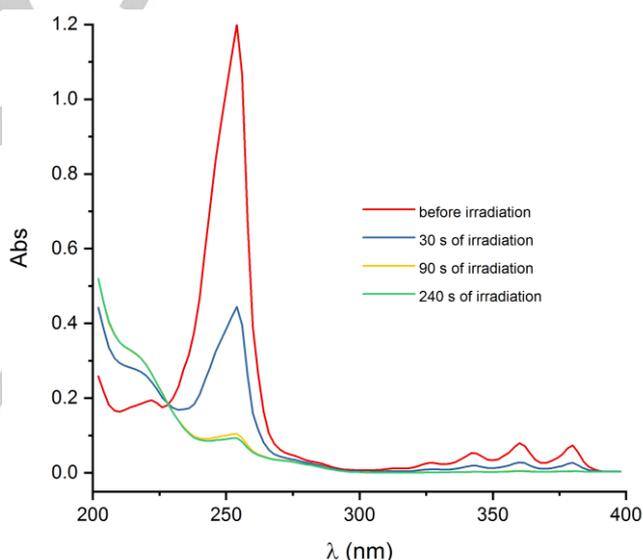
**Figure 2.** Progress of a photochemical [4+4] cycloaddition in **10** monitored by UV-Vis spectroscopy.
