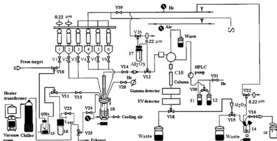
**Figure 1.** Schematic diagram of the automated synthesis of [ $^{18}\text{F}$ ]FAC using HPLC purification.
