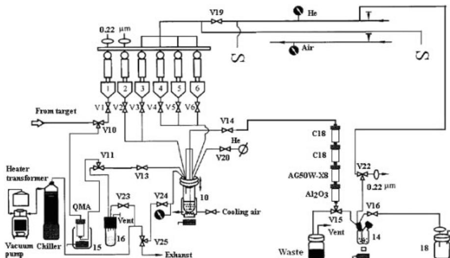
**Figure 2.** Schematic diagram of the automated synthesis of  $[^{18}\text{F}]\text{FAC}$  using on-column hydrolysis and SEP-PAK purification.
