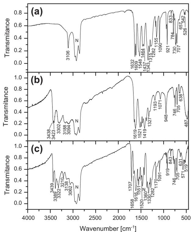
**Fig. 4.** Room temperature FTIR spectra of picric acid (a), 1-(diaminomethylene)thiourea (b) and 1-(diaminomethylene)thiuron-1-ium picrate (c).
