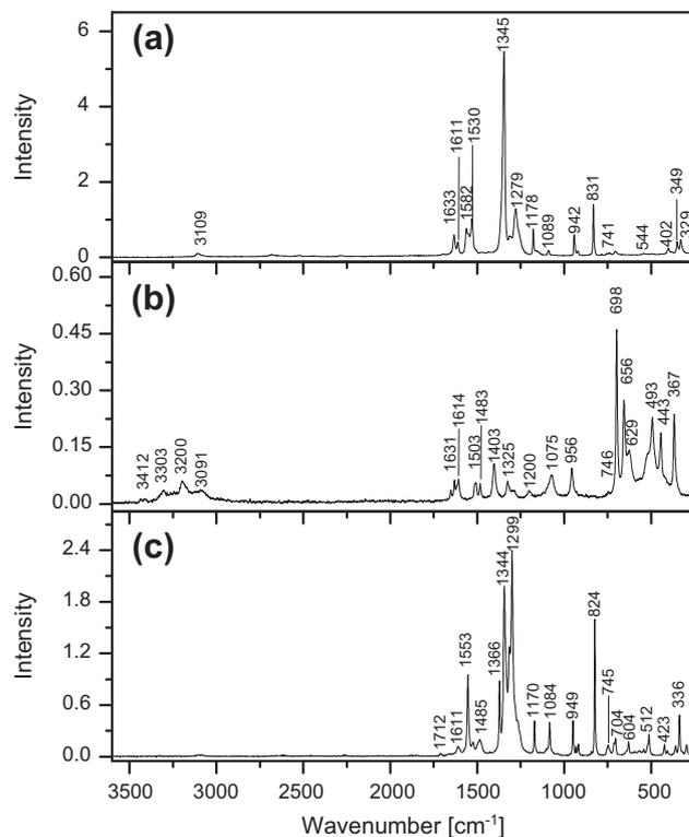
**Fig. 5.** Room temperature Raman spectra of picric acid (a), 1-(diaminomethylene)thiourea (b) and 1-(diaminomethylene)thiuron-1-ium picrate (c).
