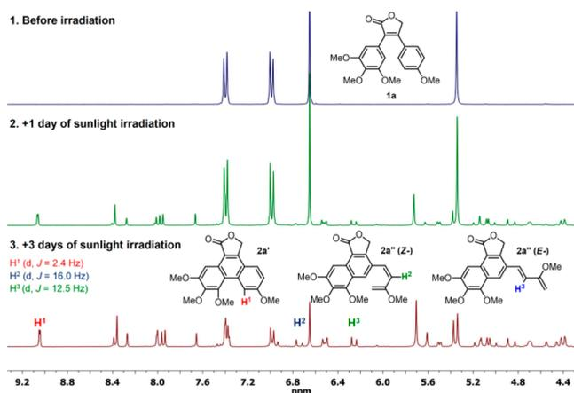
**Figure 3.**  $^1\text{H}$  NMR monitoring of diarylethene **1a** upon sunlight irradiation.
