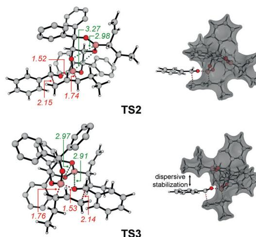
**Figure 1.** Calculated transition-state structures **TS2** and **TS3** with selected bond lengths (in Å) and side views highlighting the dispersive stabilization of **TS3**. For clarity, the hydrogens on the phenyl rings of the boronates are not shown.
