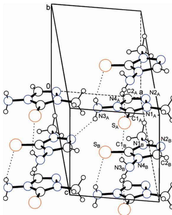
Fig. 3 (color online). Columns of two independent molecules formed by N–H...S interactions along *b* in the crystal structure of **11**.
