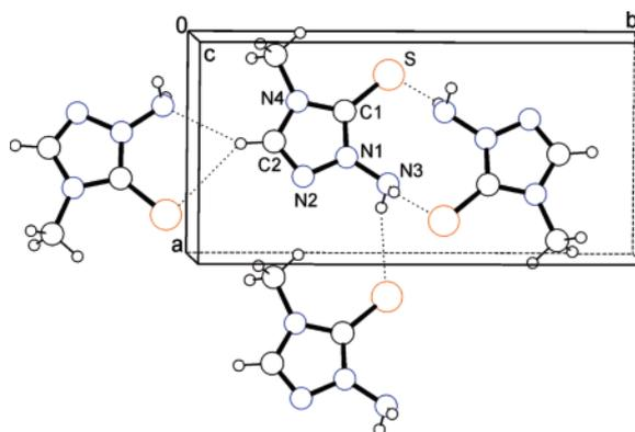
Fig. 7 (color online). Crystal structure of **15** showing N–H...S hydrogen bonds as well as bifurcated C–H...S and C–H...N contacts.
