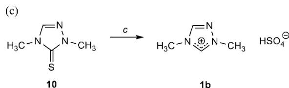
Scheme 1. a)  $\frac{1}{8}$  S<sub>8</sub>, Et<sub>3</sub>N/pyridine; b)  $\frac{1}{8}$  S<sub>8</sub>, K<sub>2</sub>CO<sub>3</sub>/MeOH; c) O<sub>2</sub>/H<sub>2</sub>O, 160 °C.
