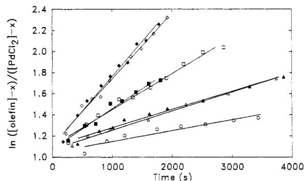
**Figure 1.** Kinetic plots for reaction of methylenecyclohexane with  $\text{Na}_2\text{PdCl}_4$  in AcOH at 60 (O), 70 ( $\Delta$ ), 80 ( $\square$ ), and 90 °C ( $\diamond$ ).
