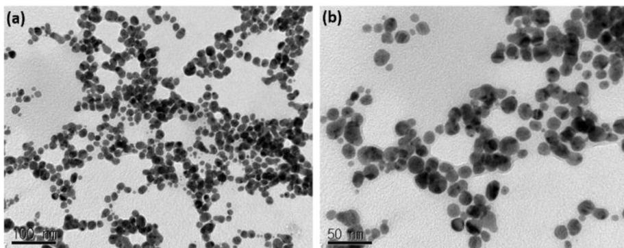
Fig. 2. TEM images of Ag NPs synthesized with *Radix Puerariae* extract. (a) With magnification 100 nm and (b) with 50 nm.
