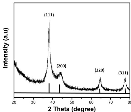
Fig. 4. The XRD spectrum of Ag NPs synthesized with *Radix Puerariae* extract.
