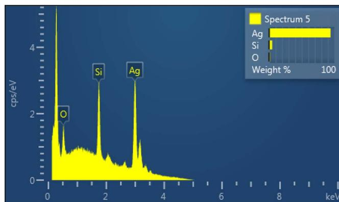
Fig. 3. The EDX spectrum of Ag NPs synthesized with *Radix Puerariae* extract.
