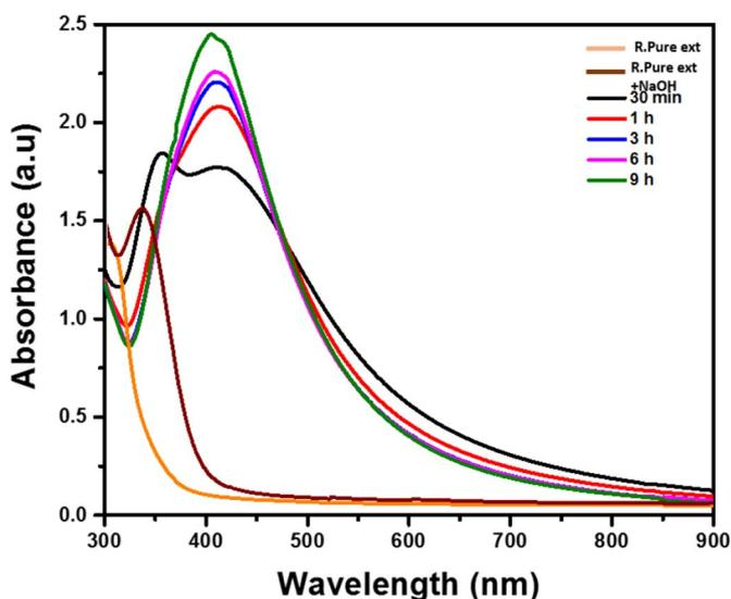
Fig. 1. UV-Vis spectra of Ag NPs synthesized with *Radix Puerariae* extract.
