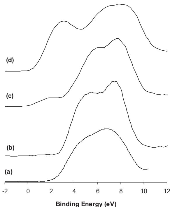
**Fig. 2.** XPS of the VB energy region after calcination at 773 K of MoTi (a), RbMoTi (b), after hydrogen reduction of RbMoTi at 473 K (c), after hydrogen reduction of RbMoTi at 673 K (d).
