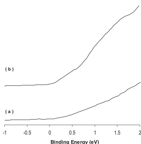
**Fig. 3.** UPS of Rb modified Mo catalyst RbMoTi after calcination at 773 K (a), after in-situ hydrogen reduction at 673 K for 12 h (b).
