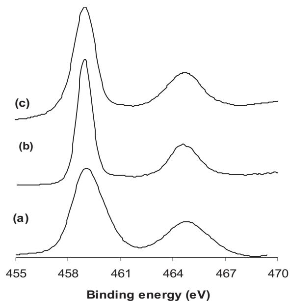
**Fig. 4.** XPS of  $\text{Ti}(2\text{p})$  energy region after calcination at 773 K of MoTi (a), RbMoTi (b), after hydrogen reduction of RbMoTi at 673 K (c).
