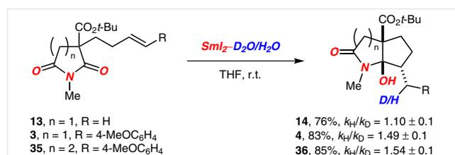
**Scheme 2** Kinetic isotope effect in the cyclization of imides to 2-azabicycles using  $\text{SmI}_2\text{-D}_2\text{O}$
