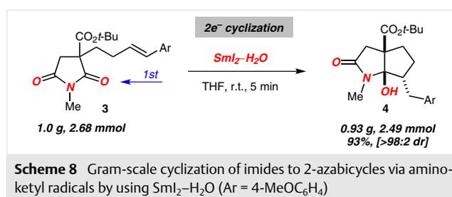
**Scheme 8** Gram-scale cyclization of imides to 2-azabicycles via aminoketyl radicals by using Sml<sub>2</sub>-H<sub>2</sub>O (Ar = 4-MeOC<sub>6</sub>H<sub>4</sub>)
