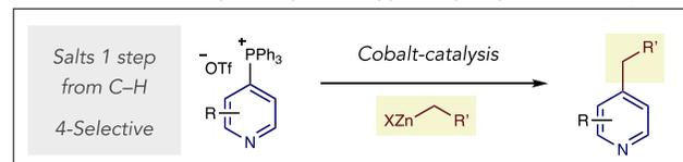
reaction pathway.<sup>7</sup> The most common methods to make alkylated pyridines are transition metal-catalyzed cross-coupling reactions between pyridyl(pseudo)halides and alkyl organometallic reagents.<sup>8</sup> These reactions are broadly effective to alkylate pyridine building blocks where halide or psuedohalides are commercially available, or can be
