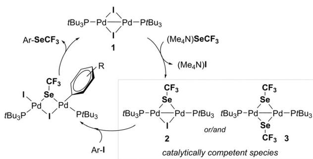
Figure 1. Anticipated Pd<sup>I</sup>-dimer catalyzed C–SeCF<sub>3</sub> coupling.
