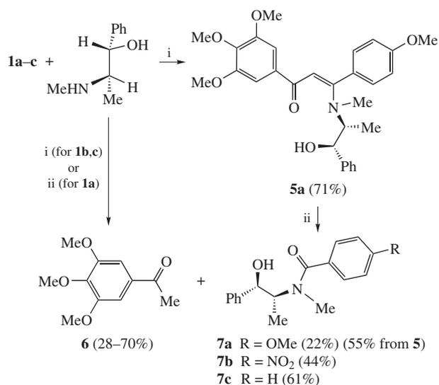
Scheme 4 Reagents and conditions: i, 1,4-dioxane, reflux; ii, CuCl, pyridine, 1,4-dioxane, reflux.
