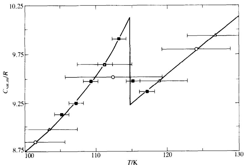
FIGURE 7. Experimental average heat capacities in the cr(III)-to-cr(II) transition region for 1,2,3,4-tetrahydroquinoline.  $\Delta$ , Series 7;  $\circ$ , series 8;  $\blacksquare$ , series 14. The horizontal bars span the temperature increment associated with each average heat-capacity value. The heat-capacity curve is described in the text.
