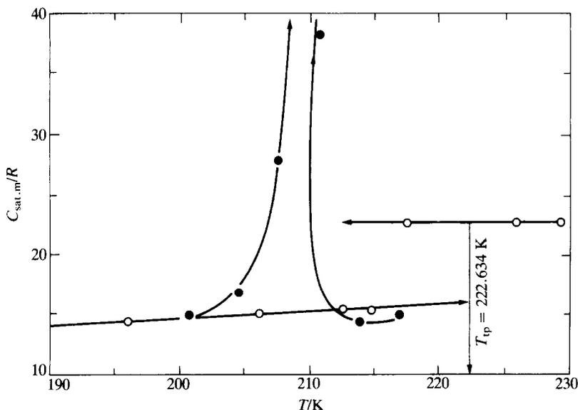
FIGURE 3. Heat capacity against temperature near the triple-point temperature for 5,6,7,8-tetrahydroquinoline.  $\circ$ , Experimental results for the stable crystal and liquid phases;  $\bullet$ , series 13 results for the metastable crystalline form. The vertical line indicates the triple-point temperature. The curves are guides for the eye.
