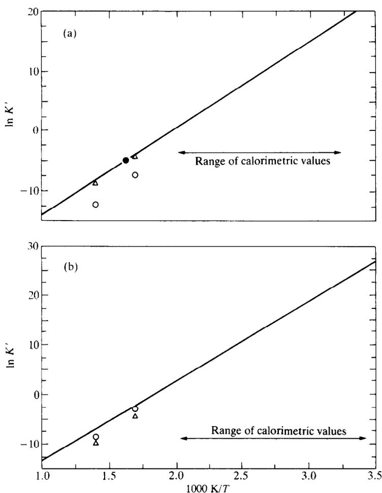
FIGURE 8. Plot of  $\ln K'$  as a function of inverse temperature for the hydrogenation of quinoline to (a), 1,2,3,4-tetrahydroquinoline and (b), 5,6,7,8-tetrahydroquinoline:  $\Delta$ , experimental (reference 11);  $\circ$ , estimated (reference 11);  $\bullet$ , reference 44. The solid lines represent the functions calculated from the calorimetric results. The lines are an extrapolation in the region 1.0 to 2.0 on the x-axis. See text for definition of  $K'$ .
