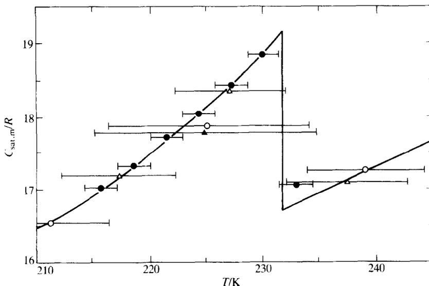
FIGURE 6. Experimental average heat capacities in the cr(II)-to-cr(I) transition region for 1,2,3,4-tetrahydroquinoline.  $\Delta$ , Series 1;  $\bullet$ , series 5;  $\circ$ , series 6;  $\blacktriangle$ , series 15. The horizontal bars span the temperature increment associated with each average heat-capacity value. The heat-capacity curve is described in the text.
