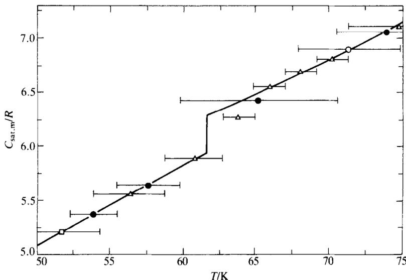
FIGURE 5. Experimental average heat capacities in the cr(IV)-to-cr(III) transition region for 1,2,3,4-tetrahydroquinoline.  $\circ$ , Series 7;  $\triangle$ , series 9;  $\bullet$ , series 11;  $\square$ , series 12. The horizontal bars span the temperature increment associated with each average heat-capacity value. The heat-capacity curve is described in the text.
