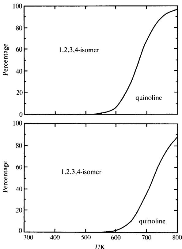
FIGURE 9. Relative percentages of quinoline and 1,2,3,4-tetrahydroquinoline at thermodynamic equilibrium in the gas phase at different temperatures. The upper chart is under a hydrogen pressure of 3.55 MPa, and the lower chart is for 7.0 MPa hydrogen pressure.
