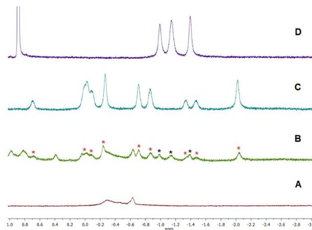
**Figure 6.** Partial <sup>1</sup>H NMR (600 MHz, D<sub>2</sub>O, 298 K) spectra of: Initial host-guest complex **10@1** (A), after addition of Ph<sub>3</sub>SnH (2 eq.), AAPH (cat.) after 12 h at 40 °C (B), authentic 2-bromononane in **1** (C) and authentic nonane in **1** (D). Partially-reduced and fully-reduced products are marked in the reaction mixture with red and black stars, respectively.
