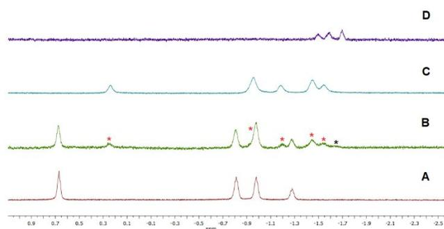
**Figure 5.** Partial <sup>1</sup>H NMR (600 MHz, D<sub>2</sub>O, 298 K) spectra of: Initial host-guest complex **8@1** (A), after addition of Ph<sub>3</sub>SnH (2 eq.), AAPH (cat.) after 12 h at 40 °C (B), authentic 1-iodoheptane in **1** (C) and authentic heptane in **1** (D). Partially-reduced and fully-reduced products are marked in the reaction mixture with red and black stars, respectively.
