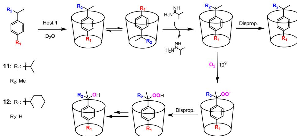
**Scheme 5.** Mechanism of aerobic oxidation of alkyl aromatic compounds (**11** and **12**) in **1**.
