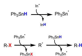
**Scheme 1.** Generation of tin radical in presence of radical initiator (Top). General mechanism for radical reduction of alkyl halides (RX where X = Br or I) using  $\text{Ph}_3\text{SnH}$  as reducing agent (Bottom).
