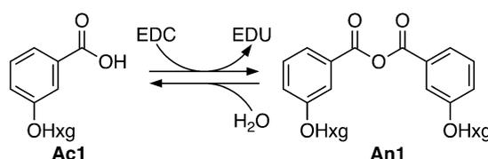
**Scheme 2.** EDC-fueled assembly of monoacid **Ac1**.
