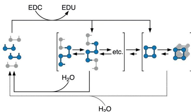
**Figure 6.** Proposed mechanism for the chemically fueled self-assembly of macrocycles in this system. Both the interconversion of the anhydrides and the difference in hydrolysis rates contribute to the efficiency.
