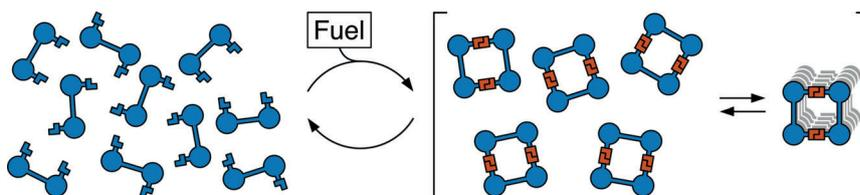
**Out-of-equilibrium assembly:** Diacid precursors assemble into unstable aqueous anhydride macrocycles on treatment with carbodiimide chemical fuels, even though initial anhydride generation is unselective
