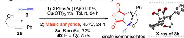
Excellent stereoselectivity was achieved for this cascade reaction with only *endo*-product obtained. The structure was confirmed by X-ray crystallography (**8b**). To evaluate the reaction scope, various homopropargyl alcohols, alkynes and dienophiles were tested as shown in **Table 2**.
