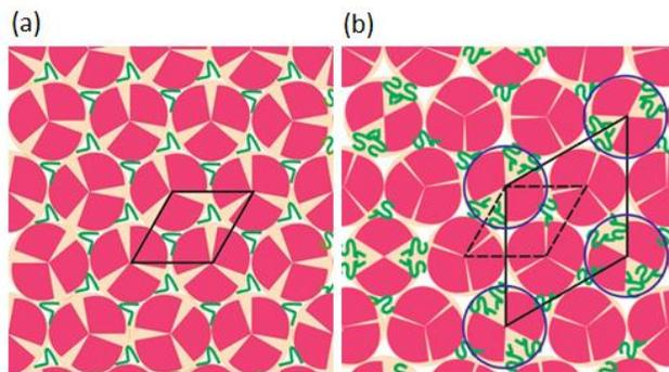
Figure 3. Schematic model of a layer of the 12-12-12Li + C19D40 80/20 blend in the (a) Col<sub>h</sub> and (b) superlattice phase (pink: minidendrons; green: n-alkane).
