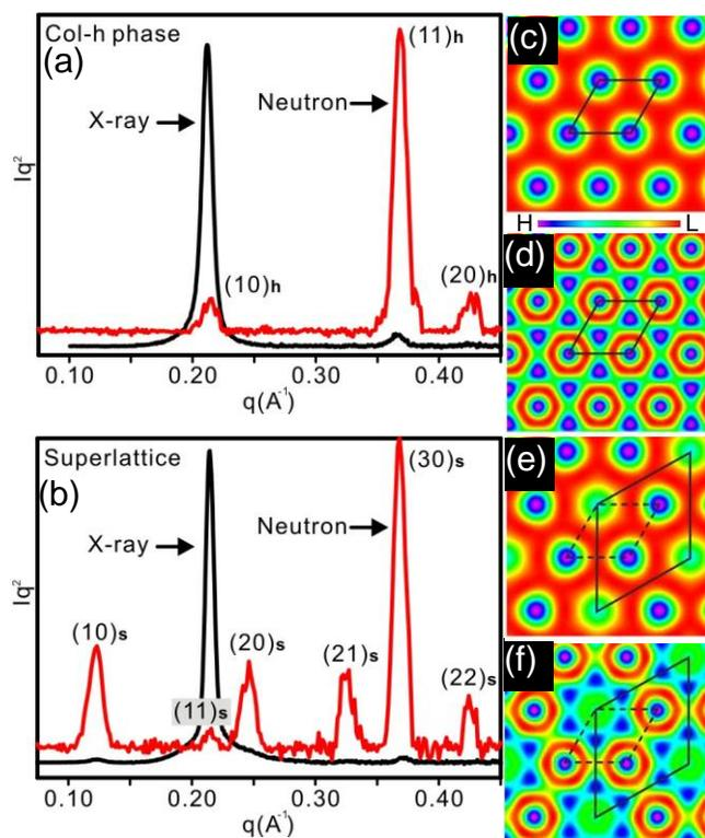
Figure 2. (a,b) Small-angle X-ray (black) and neutron powder diffractograms (red) of 12-12-12Li + C<sub>19</sub>D<sub>40</sub> 80/20 in the (a) Col<sub>h</sub> phase at 70 °C and (b) the superlattice phase at 130 °C. (c) ED and (d) neutron SLD map of the Col<sub>h</sub> phase. (e) ED and (f) SLD map of the Col<sub>s</sub>. Neutron experiments at station D16 at ILL, Grenoble.
