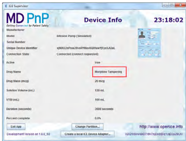
Figure 9: The tampered message displayed on the ICE Supervisor front panel.
