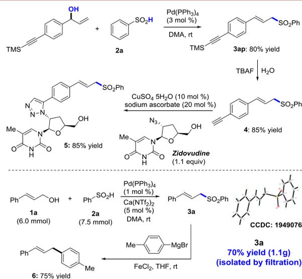
**Figure 3.** Utility of this protocol and synthetic transformation of allylic sulfones.
