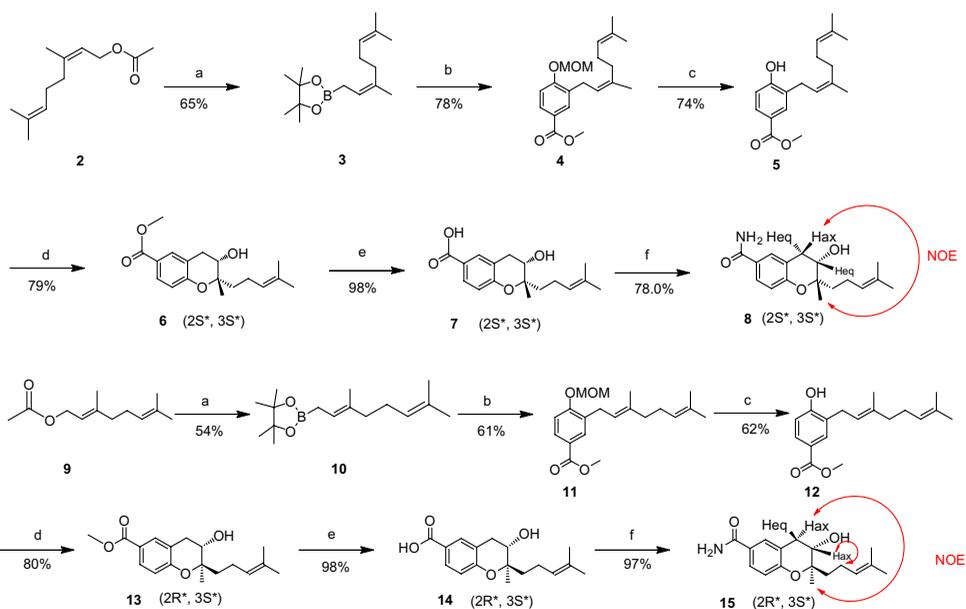
**Scheme 2.** Synthesis of racemic xiamenmycin C. Reagents and conditions: (a)  $B_2Pin_2$ ,  $Ni(cod)_2$ ,  $PCy_3$ ,  $AcOEt$ ; (b) methyl 3-bromo-4-hydroxybenzoate,  $Pd(dppf)Cl_2$ ,  $CsCO_3$ , 1,4-dioxane; (c) D-camphorsulfonic acid,  $MeOH$ ; (d)  $VO(acac)_2$ ,  $TBHP$ ,  $TFA$ ,  $DCM$ ; (e) 4 N  $NaOH$ ,  $CH_3OH$ ; (f)  $Boc_2O$ , pyridine,  $NH_4HCO_3$ , 1,4-dioxane.
