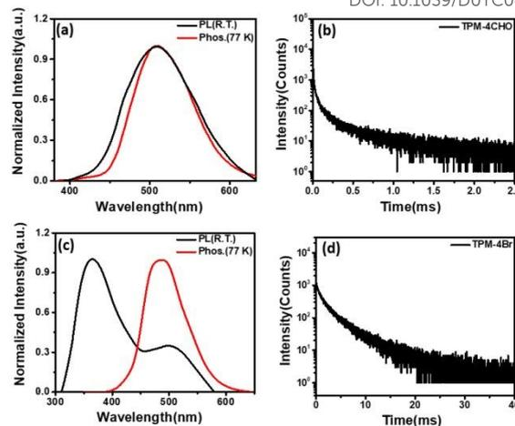
**Fig. 2** (a) Steady-state spectra (room temperature), delay spectra (77 K, delay time: 50 ms) and (b) Lifetime decay curve of TPM-4CHO in crystal at room temperature. (c) Steady-state spectra (room temperature), delay spectra (77 K) and (d) Lifetime decay curve of TPM-4Br in crystal at room temperature.
