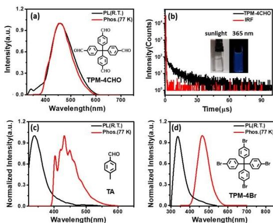
**Fig. 1** Steady-state spectra (room temperature in deaerated THF) and delay spectra (77 K, delay time: 10 ms) of (a)TPM-4CHO, (c)TA and (d)TPM-4Br in THF. (b)Lifetime decay curve of TPM-4CHO at room temperature in deaerated THF and instrument response function (IRF). Insets in b show photographs of TPM-4CHO upon sunlight (left) and under 365 nm UV-light (right) in deaerated THF at room temperature.
