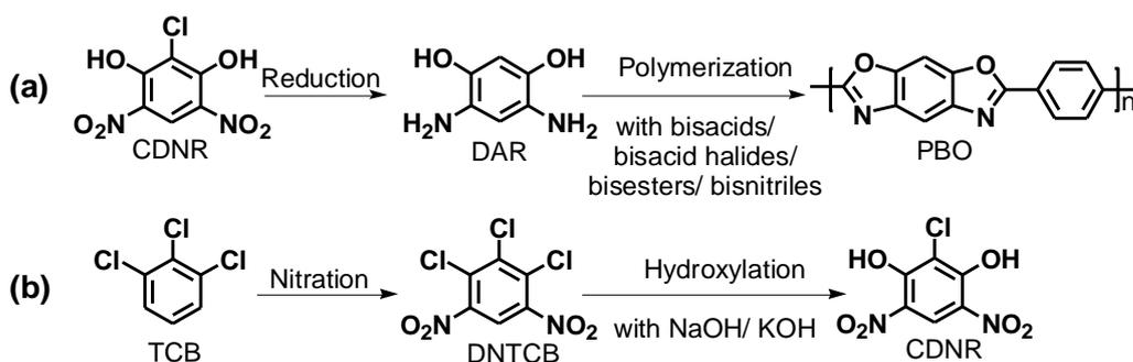
**Scheme 1.** (a) Synthesis of PBO fibers from DAR, which can be obtained from CDNR, and (b) synthesis of CDNR from DNTCB, obtained from nitration of TCB.
