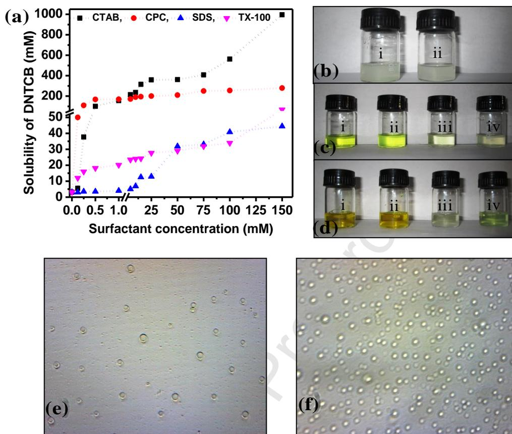
**Figure 4.** (a) Solubility of DNTCB in different micellar solutions, (b-d) Color of DNTCB solubilized micellar solutions [(b) 0.5 mM, (c) 15 mM, (d) 100 mM; i: CTAB, ii: CPC, iii: SDS, iv: TX-100], (e & f) optical microscope images of DNTCB-0.5 mM CPC and DNTCB-0.5 mM CTAB emulsion solutions, respectively.
