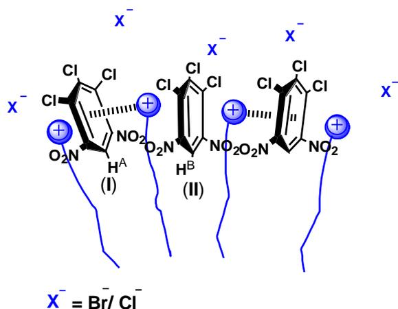
**Scheme 3.** DNTCB molecules in cation- $\pi$  interaction with surfactant's cationic head group (structure **I**), and hydrophobically solubilized (structure **II**) in micellar phase of cationic (CTAB/ CPC) micelles.
