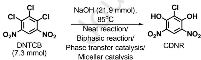
**Scheme 2.** Reaction of DNTCB with NaOH to synthesize CDNR under different conditions.
