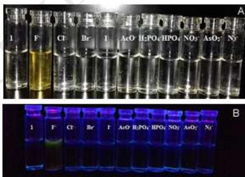
**Fig. 5.** Colorimetric changes of compound **1** ( $9 \times 10^{-4}$  M) in acetonitrile in presence of  $15 \times 10^{-4}$  M anions A: naked eye B: under UV light at 366 nm.
