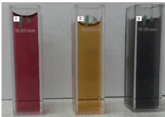
**Fig. 5.** Color change of solutions during the formation of the **Co-3OHPP-nAu** complex. Red gold colloid (1); yellow **Co-3OHPP** (2); violet-blue gold-porphyrin complex (3).
