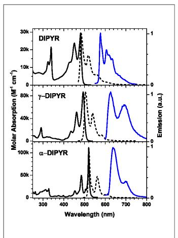
Figure 3. Absorption (solid) and normalized fluorescence (dashed) and phosphorescence (blue) spectra recorded in methylcyclohexane; left axis is molar absorbance; right axis is normalized emission intensity.
