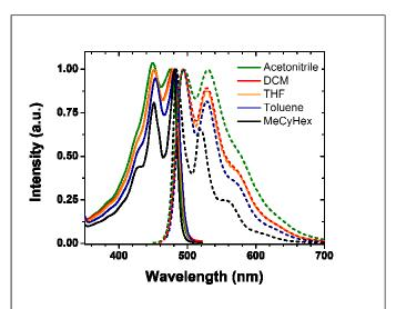
**Figure 4.** Normalized absorption (solid) and emission (dashed) spectra of DIPYR in solvents of increasing polarity. Note that the relative intensity of the 0-1 vibronic feature increases with increasing polarity, suggesting the presence of a second, underlying absorptive feature which
