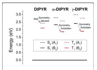
**Figure 6.** Intersystem crossing from  $S_1$  to  $T_2$  occurs rapidly in DIPYR, as the process is both exergonic and symmetry-allowed. In  $\alpha$ - and  $\gamma$ -DIPYR, however, the only exergonic ISC mechanism is symmetry forbidden, and thus occurs too slowly to compete with fluorescence.
