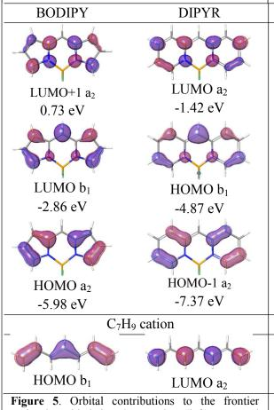
**Figure 5**. Orbital contributions to the frontier molecular orbitals in BODIPY dyes (left) compared with DIPYR dyes (right).
