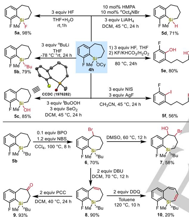
**Figure 4.** Synthetic applications of sila-benzosuberane **4h**.
