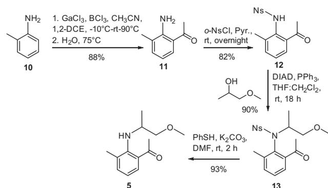
Scheme 2. Synthesis of intermediate **5** by a Mitsunobu alkylation of nosyl-activated aniline.
