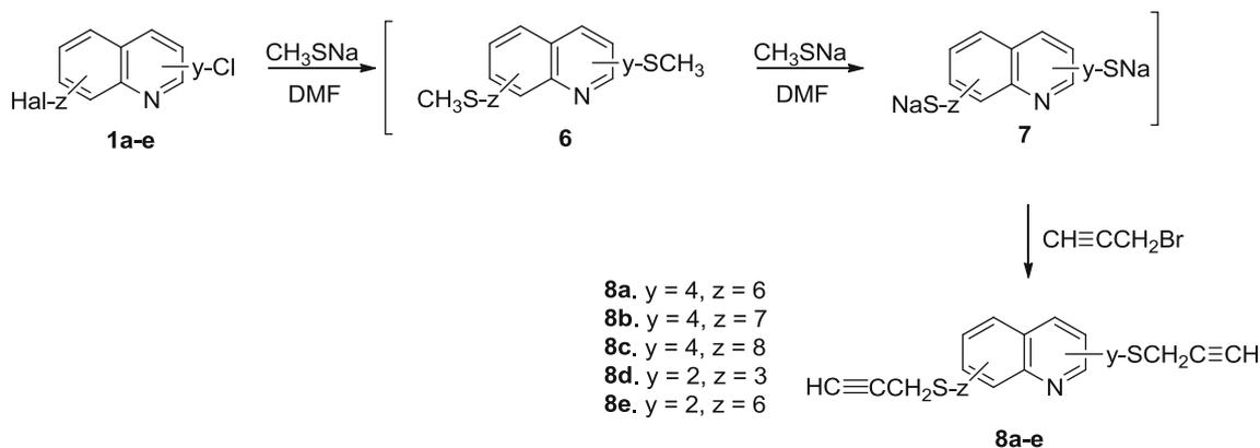
**Scheme 2** Synthesis of dipropargylthioquinolines **8a–e**
