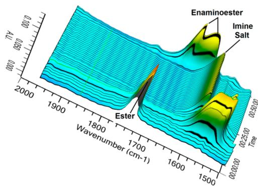
Figure 2. ReactIR of saturated cyanoester reduction (24).
