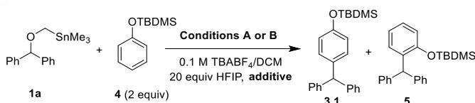
**Conditions A:** I = 2.5 F/mol, 20 mA, graphite electrodes, r.t., 40 min
