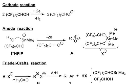
**Figure 2.** Proposed mechanism of electrochemically induced Friedel-Crafts reaction.
