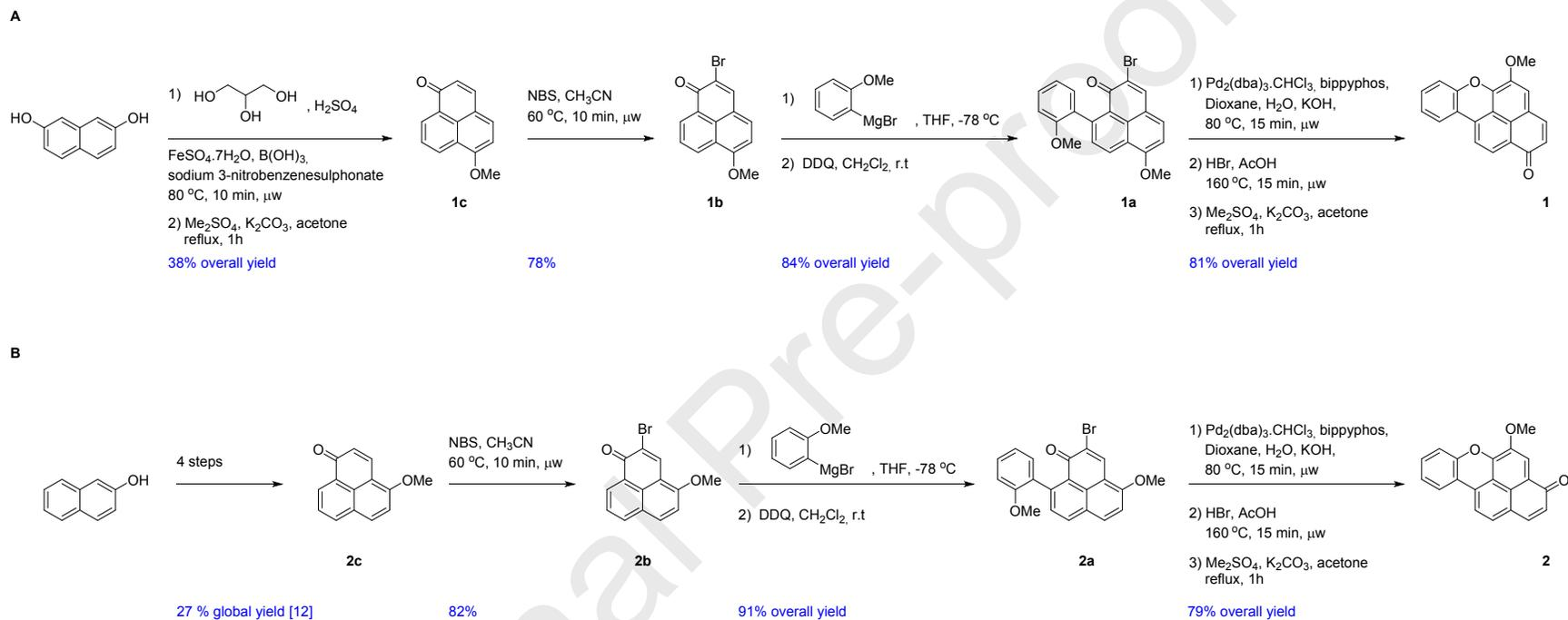
**Scheme 2:** Synthesis of compounds **1** (part **A**) and **2** (part **B**) starting from the corresponding methoxyphenalenones **1c** and **2c**.
