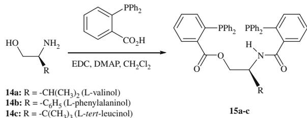
**Scheme 3.** Synthesis of  $\beta$ -benzoyloxybenzamides **15a–c**.
