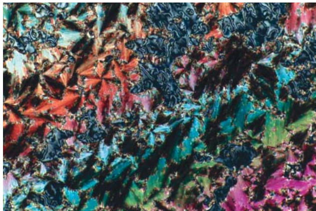
Fig. 1 S_C phase of compound 39 at 127.1 °C clearly showing broken focal conic domains accompanied by regions of pseudohomeotropic schlieren texture (100 \times magnification).
