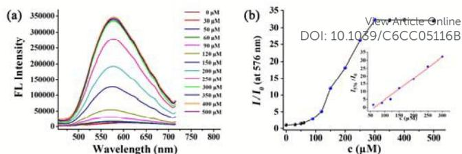
**Figure 2.** (a) Fluorescence spectra of the TPE-DABF complex (TPE-DABA, 50  $\mu\text{M}$ ; D-fructose, 30 mM) upon titration of  $\text{H}_2\text{O}_2$ . (b) Plot of the relative fluorescence intensity ( $I/I_0$ ) at 576 nm versus the concentration of  $\text{H}_2\text{O}_2$ . Inset: linearity of the ratio of fluorescence intensity ( $I/I_0$ ) at 576 nm.  $\lambda_{\text{ex}}$  = 430 nm.
