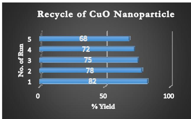
Figure 5. Recycle of catalyst CuO nanoparticle
