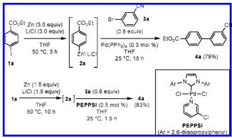
organometallics have, however, the drawback of being air- and moisture-sensitive. Recently, we have developed a very efficient LiCl-mediated direct insertion of zinc into unsaturated halides.<sup>5</sup> Using this method, we wish to report a one-pot protocol avoiding the handling of sensitive organozinc intermediates.
