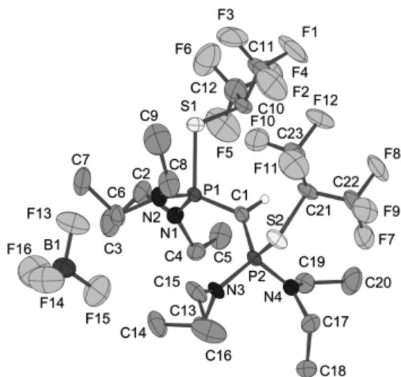
Figure 3. Perspective view and labeling scheme for the molecule **18**; selected bond lengths [pm] and angles [°]: P(1)–N(1) 163.6(3), P(1)–C(1) 169.6(4), C(1)–P(2) 169.7(4), P(1)–S(1) 212.72(14), S(1)–C(10) 182.5(4), N(1)–C(2) 148.2(5), C(10)–C(11) 152.2(6); C(1)–P(1)–N(2) 116.21(19), C(1)–P(1)–S(1) 111.42(14), N(1)–P(1)–S(1) 107.61(13), N(1)–P(1)–N(2) 108.99(17), P(1)–C(1)–P(2) 129.2(2), P(1)–S(1)–C(10) 111.86(15)
