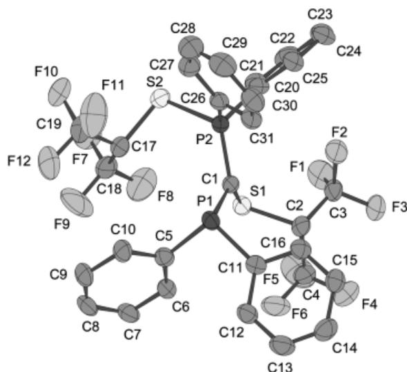
Figure 4. Perspective view and labeling scheme for the molecule **21**; selected bond lengths [pm] and angles [°]: P(1)–C(1) 181.4(5), C(1)–P(2) 170.4(5), P(2)–S(2) 215.55(19), C(1)–S(1) 176.8(5), P(1)–C(5) 183.1(5), P(2)–C(20) 181.3(5); P(1)–C(1)–P(2) 117.6(3), C(1)–P(1)–C(5) 106.2(2), P(1)–C(1)–S(1) 125.5(3), P(2)–C(1)–S(1) 113.4(3), C(1)–P(2)–S(2) 117.22(18), C(1)–P(2)–C(20) 116.0(2)
