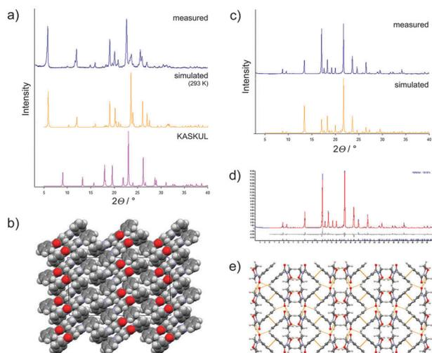
**Fig. 1** (a) Measured and simulated PXRD patterns of diamide **4**; (b) crystal packing of succinamide **4**  $\beta$ -form (view down the  $b$ -axis); (c) measured and simulated PXRD patterns of amide **6a**; (d) Rietveld plot for **6a** (blue – measured, red – calculated, grey – difference); (e) arrangement of **6a** molecules in the crystal structure (view down the  $c$ -axis).
