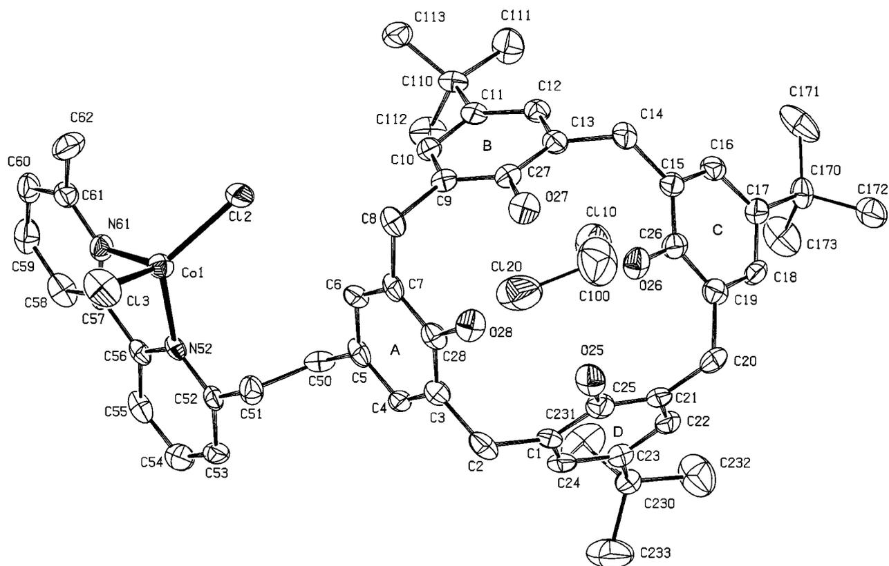
Figure 2. Numbering scheme and ORTEP underside-view of complex **13**
