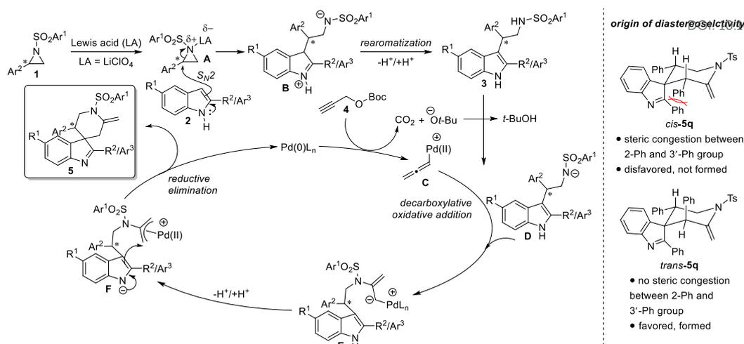
**Scheme 7.** Plausible mechanistic pathway for the synthesis of 3-spiropiperidino indolenines from activated aziridines via ring opening with 1H-indoles followed by dearomatizing spirocyclization with propargyl carbonate.
