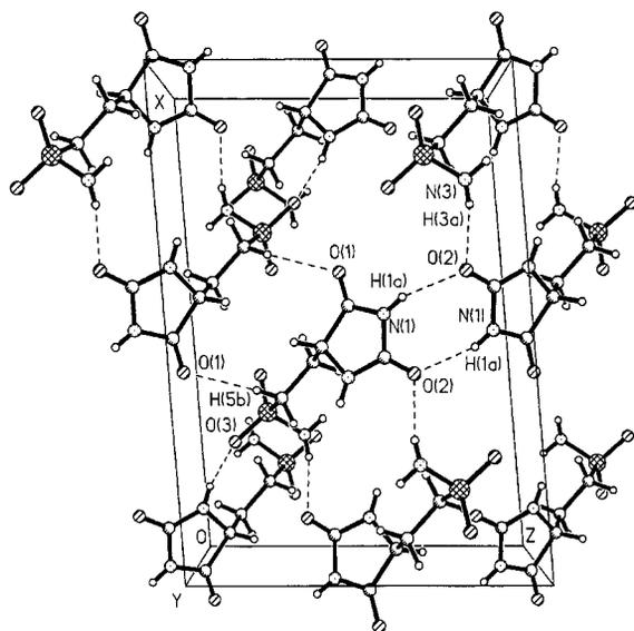
**Fig. 2.** A representation of the molecular packing arrangement in the unit cell illustrating the network of intermolecular interactions.
